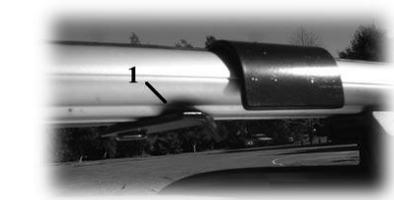
1. Swing lock bar underneath the roof rack so it is perpendicular with the bracket.
